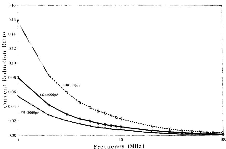
Fig. 12. Ratio of the current through the human body to the object short-circuit current for three objects having different capacitance to ground.
